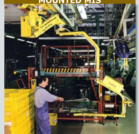
OVERHEAD TROLLEY MOUNTED MIS
